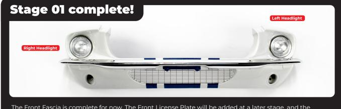
The Front Fascia is complete for now. The Front License Plate will be added at a later stage, and the assembly will connect to the rest of the body, also at a later stage.
